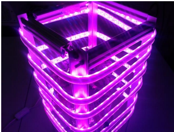
Figure 7. Using flexible LED strips for cultivation of Microtina and Vreudgenhil tomato plants from the EDEN ISS laboratory, German Aerospace Center (© Schlacht, DLR, Bremen Germany 16 March 2016)
